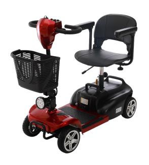
Model: MED1-KY160-B back height: 25 cm Handle width: 45 cm Overall Width: 50 cm Seat depth: 38 cm total length: 115 cm
