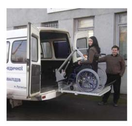
Model: ΠΠΗ-Α (Γ) Control type: Electric lift type: lifting platform
